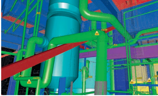
The automated Pipe Run feature lets users select points on connected, straight pipe sections, and the system automatically models a best fit pipe run with elbows in seconds.
